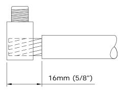
2. INSERT CONDUCTORS INTO CORRECT HOLES AND TORQUE AS SHOWN:
