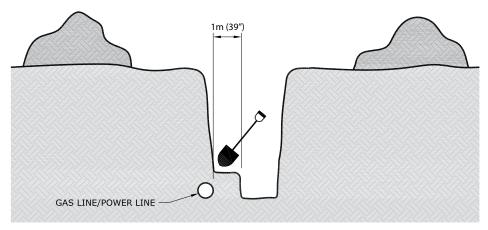
Dig a trench or bell hole 1 metre (39 inches) from the line location, parallel to the line, then hand dig laterally to expose the line.
