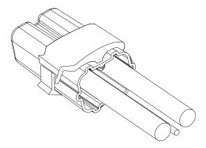
7. TO REMOVE, INSERT SCREWDRIVER BETWEEN THE CLOSING TABS AND TWIST TO OPEN THE CLAMP. REMOVE CAP SLOWLY FROM CONNECTION ALLOWING GEL TO REMAIN IN CAP.
