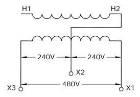
SECONDARY VOLTAGE 240/480V GROUNDED. SINGLE-PHASE PAD-MOUNTED TRANSFORMER AS SUPPLIED BY MANUFACTURER
